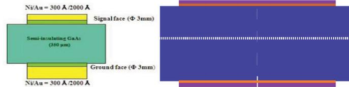
Figure 3: Cross section of the detector; after the detector is defined and displayed in 2D GVIEW
