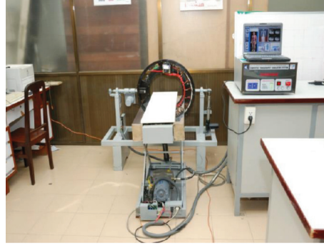
Fig.1: Model simulation computer tomography system multi-slice
