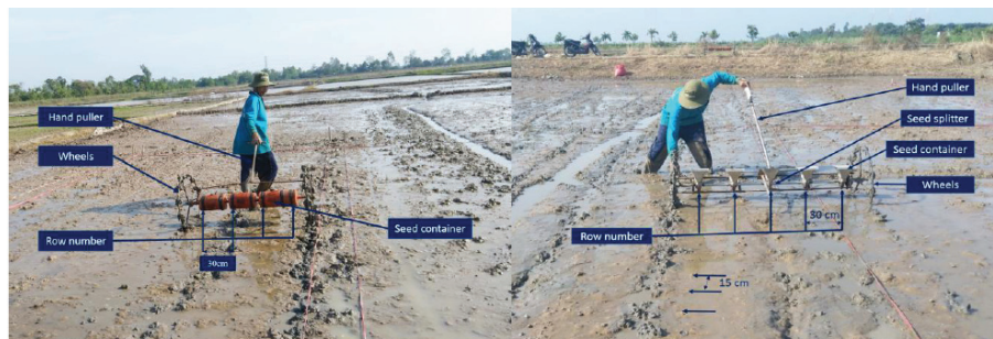
Fig. 1 The machine for drilling sowing Fig. 2 The machine for dibbling sowing
