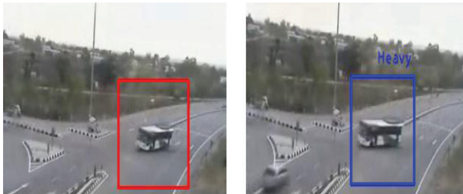
Fig. 8. (a) Vehicle detected, and (b) vehicle classified as heavy
